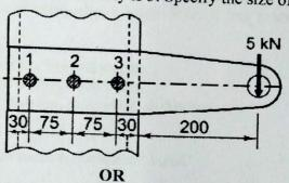
A gearbox weighing 7.5 kN is provided with a steel eye bolt for lifting and transporting on the shop-floor. The eyebolt is made of plain carbon steel 30C8 ( $S_{yt} = 400 \text{ N/mm}^2$ ) and the factor of safety is 5. Determine the nominal diameter of the eye bolt having coarse threads.
