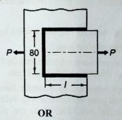
A bracket, as shown in Fig. below is welded to a plate. The welds have the same size, and the permissible force per mm of the weld-length is 1 kN. Calculate the lengths l<sub>1</sub> and l2.
