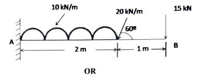
Draw the SFD (Shear Force Diagram) and BMD (Bending Moment Diagram of the Cantilever Beam as shown the in figure.
